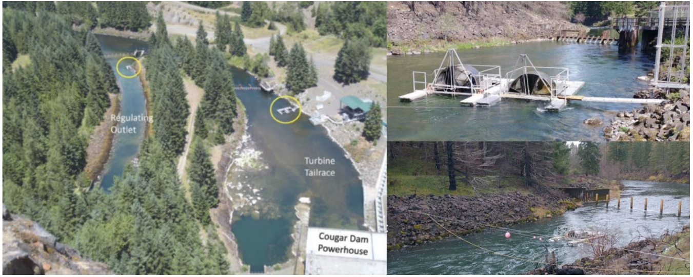
Figure 26. Cougar Dam Tailrace depicting rotary screw trap (RST) deployment locations in the powerhouse (PH) and Regulating Outlet (RO) channels. Upper right photo shows the two 8 foot diameter RSTs deployed in the PH channel in 2021. Bottom right photo shows the 5 foot diameter RST in the RO channel. The Cougar Dam spillway gates and diversion tunnel were not used during this period and therefore not represented herein.
