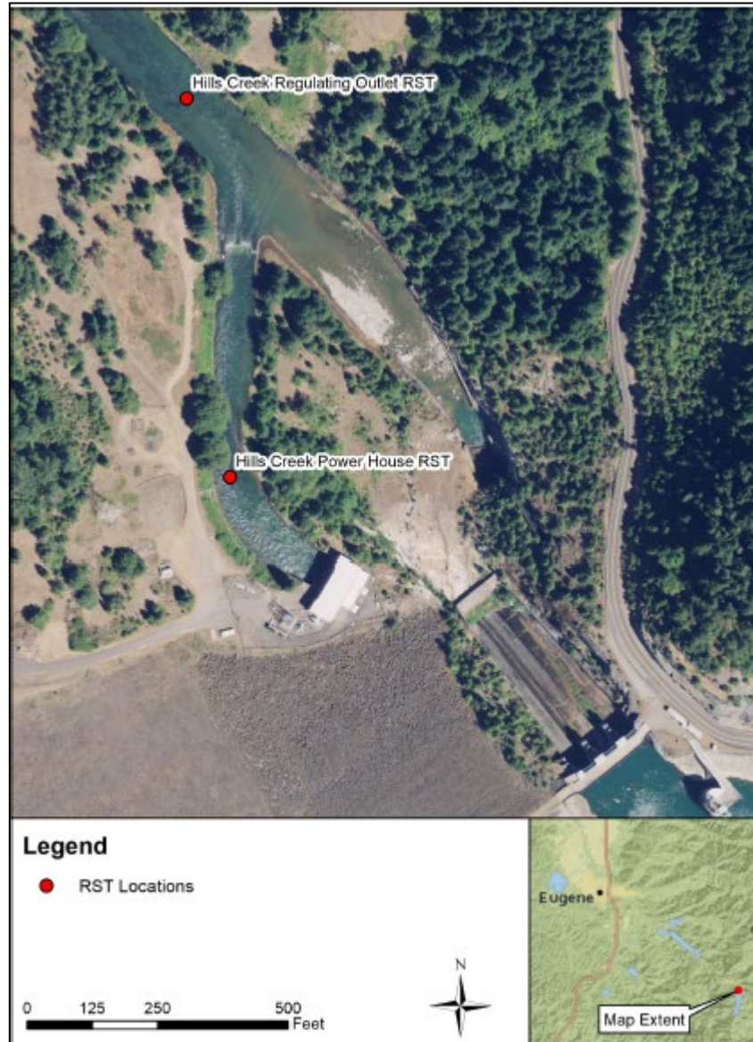
Figure 33 - Hills Creek Dam tailrace rotary screw trap sampling locations. A 5-foot diameter rotary screw trap was placed below the Regulating Outlet (RO) and an 8-foot rotary screw trap was placed below the Powerhouse (PH). A rotary screw trap was not explicitly placed/sampled below the spillway gates as the Hills Creek Dam spillway gates are only used in emergency situations and did not operate during this period.
