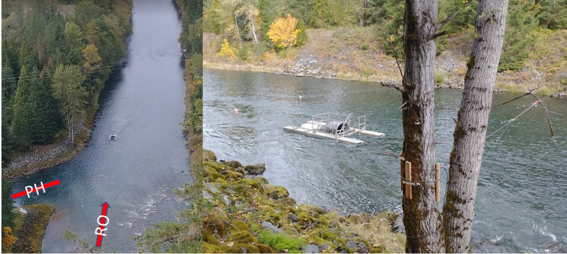
Figure 34. Hills Creek Dam – 5 foot diameter rotary screw trap below regulating outlet. Photo taken 04 September 2021 midday while powerhouse (PH) is in operation with no flow through regulating outlet (RO).
